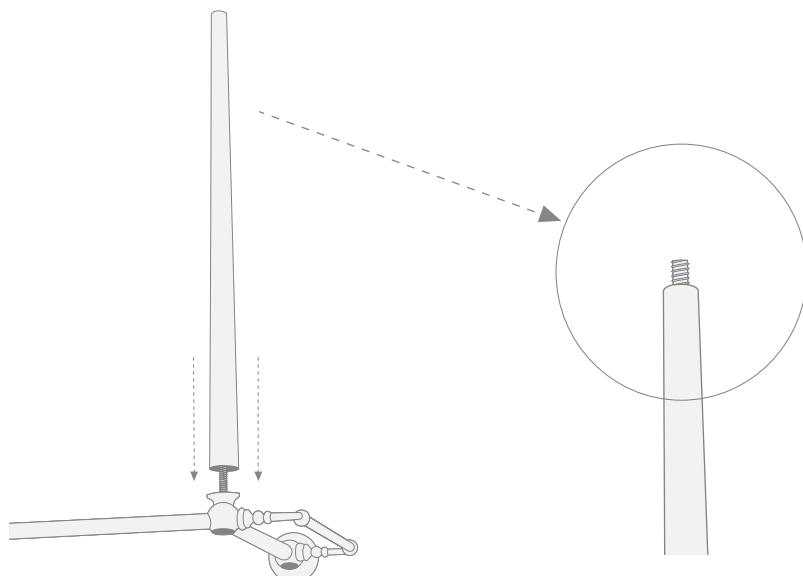
*The threaded rod should protrude slightly compared to the leg.*
