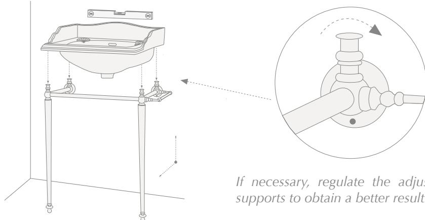
*If necessary, regulate the adjustable supports to obtain a better result.*
