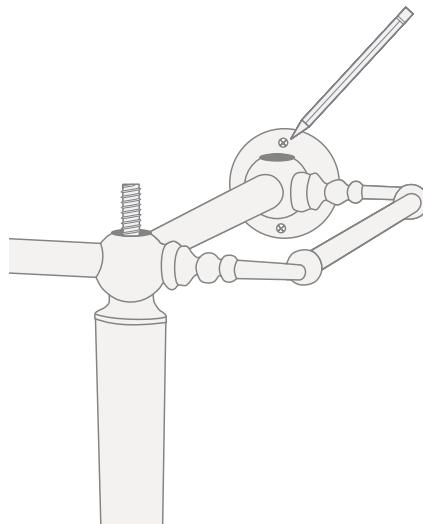
**7)** Remove the structure and make the 4 holes according to your markings.
