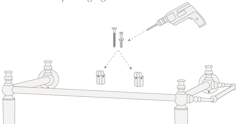
**14)** Position the basin once again, inserting the back part between the brackets and the wall.
