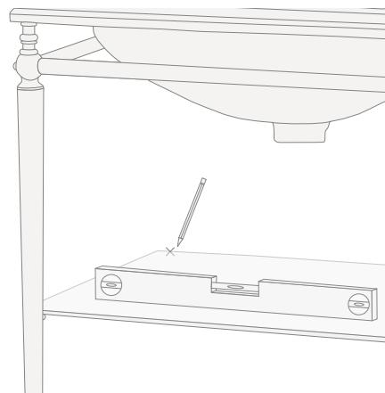
**16)** Remove the shelf, make the holes for the supports in the wall, insert the rawlplugs (I) into the wall. Assemble the supports and, last of all, the shelf.
