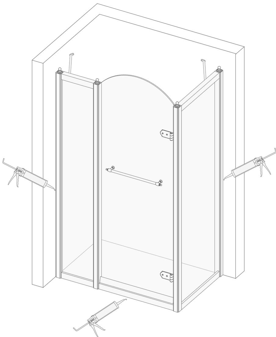
**33)** Using a piece of paper and alcohol, carefully clean off all the excess silicone around the corner enclosure.
