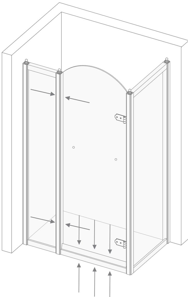
**18)** With the door perfectly adjusted, it is now possible to position the screws (H) and pre-drill the upright of the other fixed side (B) of the shower door with an iron bit ( $\varnothing$  2.5 mm).
