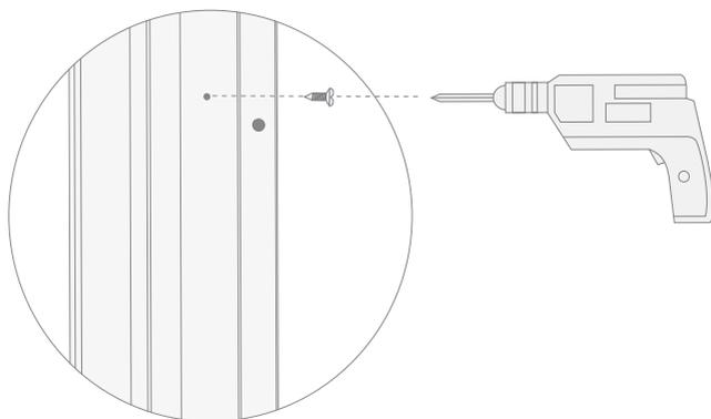
**19)** Position the plugs supplied (L: either white or black, as preferred) to cover the holes where the self-tapping screws were inserted.
