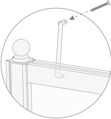
**25)** Fasten the rod with the washer (I), screw (H) and stopper (L) to the column.
