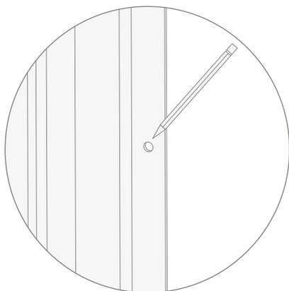
**7)** Remove the shower door and drill a hole into each of the points already marked out.
