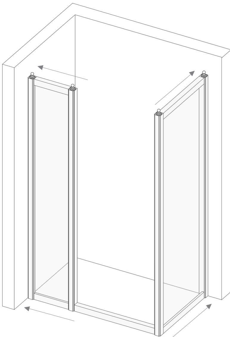
**13)** Position the screws (H), pre-drill with an iron bit ( $\varnothing$  2.5 mm) the upright of the fixed side of the shower door (E).
