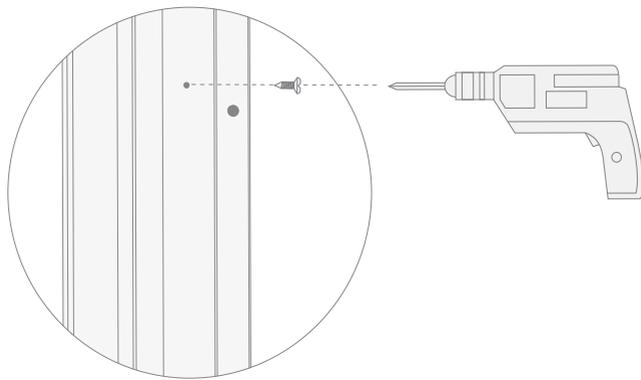
**14)** Position the supplied plugs (L: choose between black and white) to cover the holes where the self-drilling screws are inserted.
