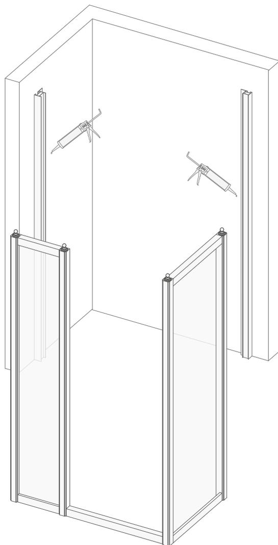
**10)** Fix the shower door to the walls with the supplied steel screws (F) until it is firmly fixed to the walls.
