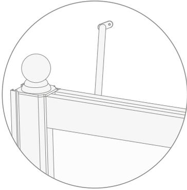
**21)** Using a pencil, mark out the two points where the rod will be positioned, on the wall and column.
