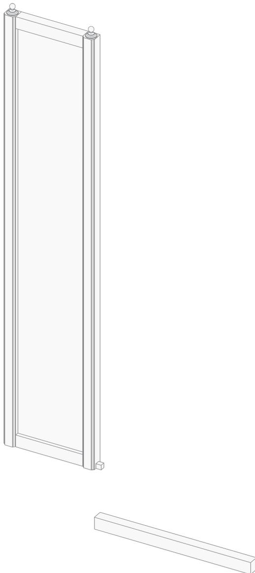
**3)** With the supplied screw, fasten the toe-kick to the fixed side of the shower door (in the point illustrated below).
