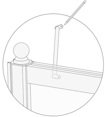
**22)** Drill a hole into the wall using the wall bit (point A) and into the upper column of the fixed side (point B) using the iron bit.
