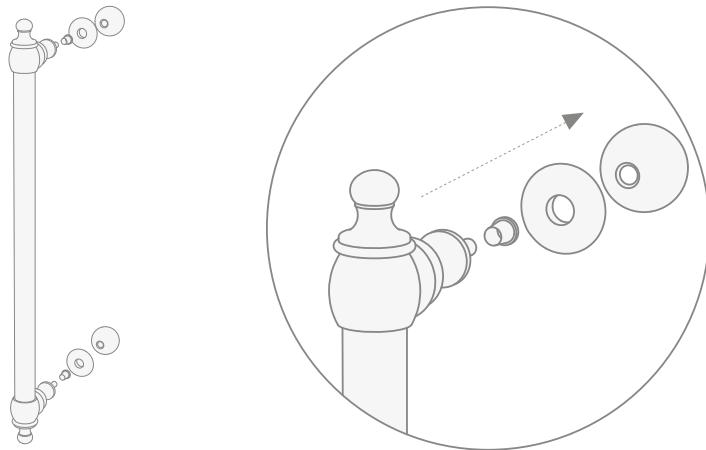
**15)** Insert the first handle (H) into the holes on the glass pane of the first shower enclosure.
