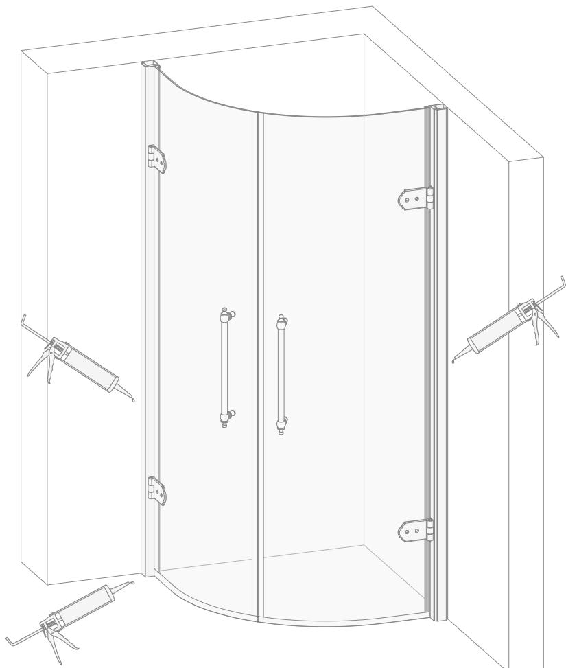
**20)** Using a piece of paper and alcohol, carefully clean off all the excess silicone around the shower enclosure.
