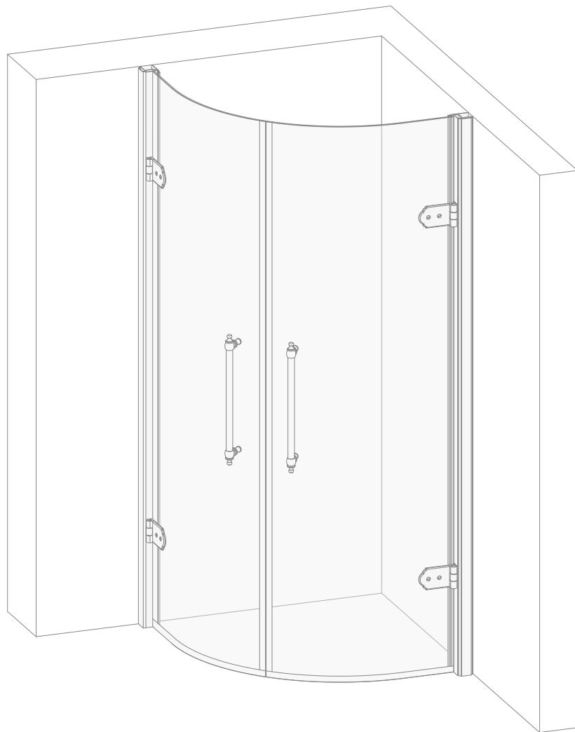
**19)** At this point, if necessary, use the silicone to seal the aluminium section bars onto the walls and shower enclosure, from the outside only.
