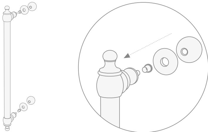
**17)** When correctly positioned, the handle should look the same as in the illustration.
