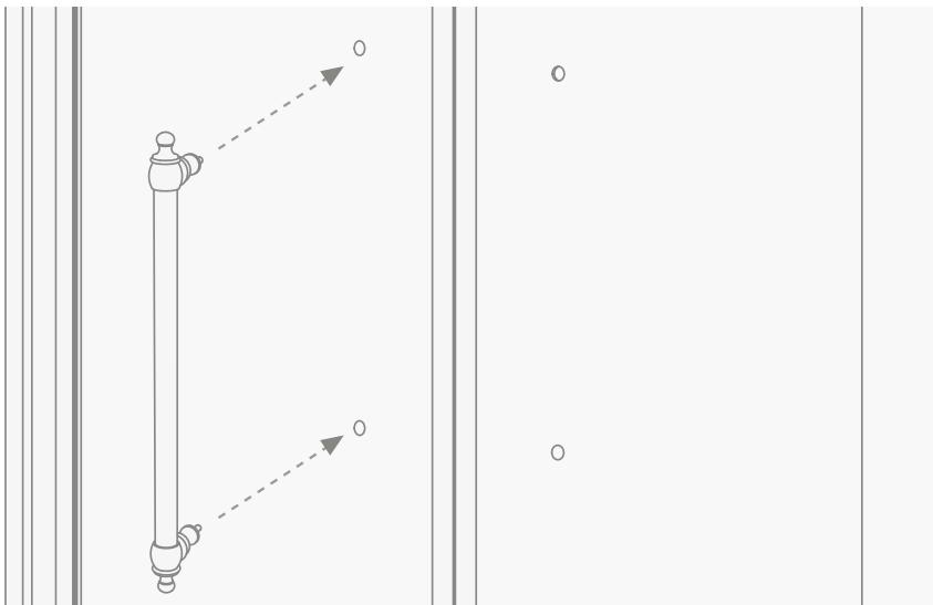
**16)** You can now fix the handle, from the inside, by screwing the parts unscrewed before from both parts back in.
