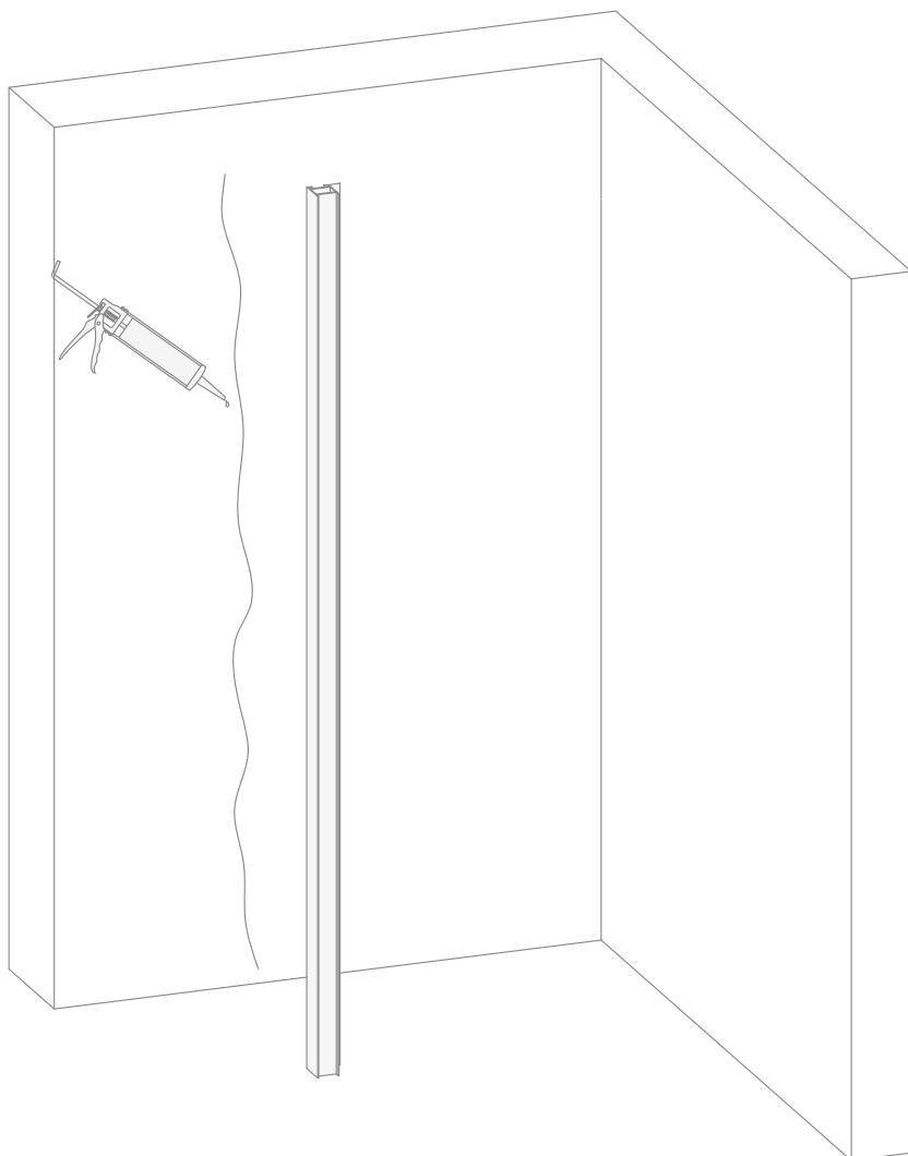
**7)** Screw the wall profile (A) to the wall with the steel screws provided (C) until firmly secured to the wall.
