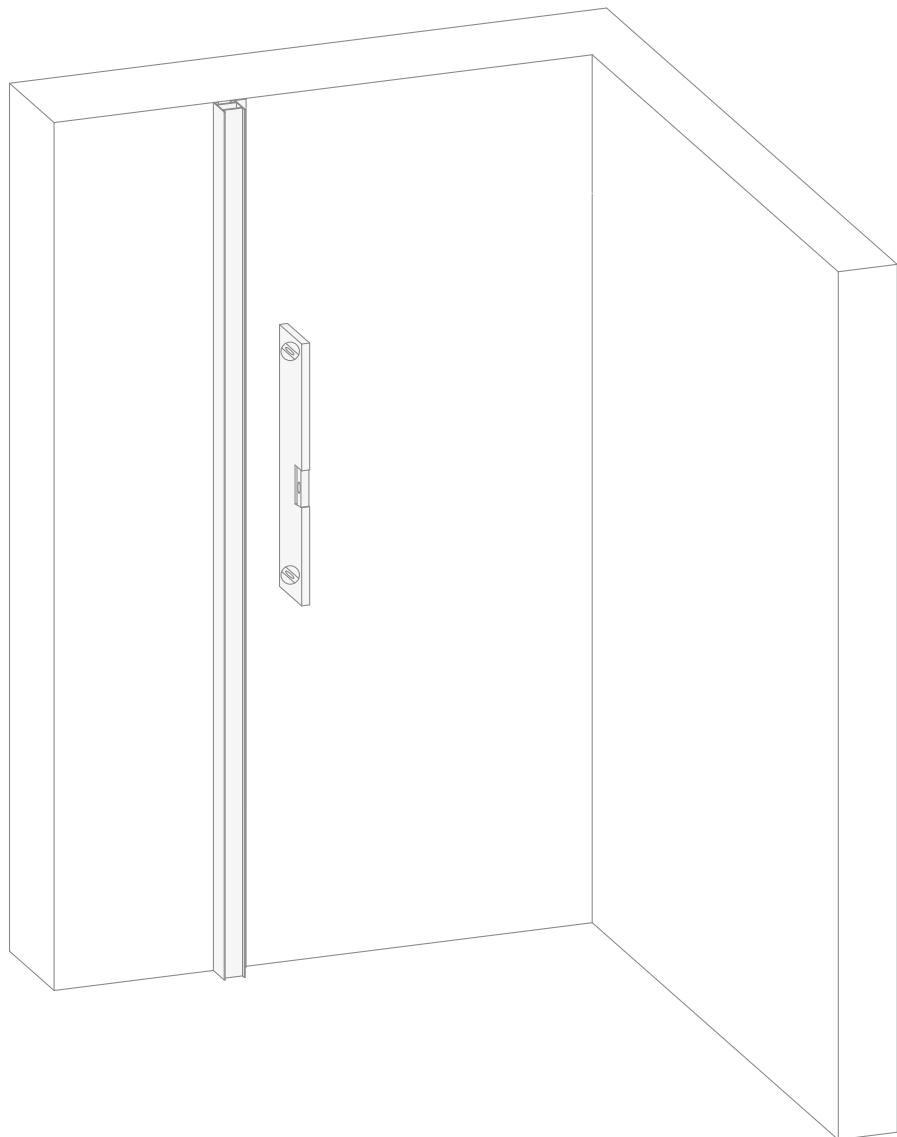
**3)** Using a pencil, mark out the two points (top and bottom) inside the profile compensator.
