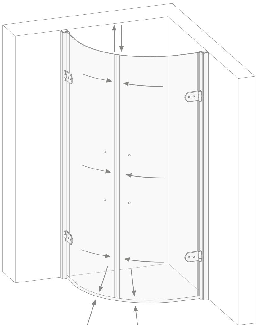
11) Using an iron drill bit, predrill the upright of the first door of the screen at two points, one at the top and one at the bottom.
