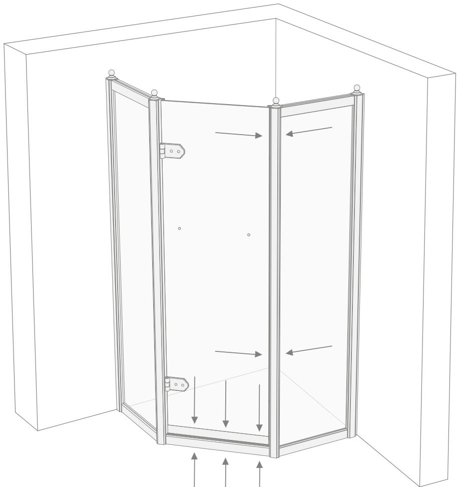
**18)** With the door perfectly adjusted, it is now possible to position the screws (G) and pre-drill the upright of the other fixed side of the shower door with an iron bit ( $\varnothing$  2.5 mm).
