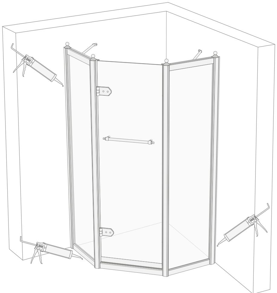
**33)** Using a piece of paper and alcohol, carefully clean off all the excess silicone around the corner enclosure.
