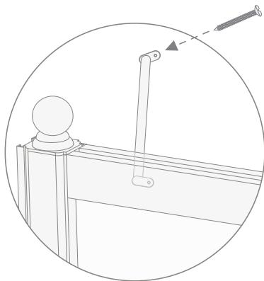
**25)** Fasten the rod with the washer (G), screw (F) and stopper (H) to the column.
