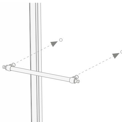
**30)** You can now fix the handle, from the inside, by screwing the parts unscrewed before from both parts back in.
