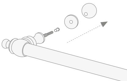
**29)** Insert the handle (M) into the holes on the glass pane of the shower enclosure.
