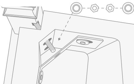
*Make sure that the threaded bar goes through the slot on the metal bracket.*
