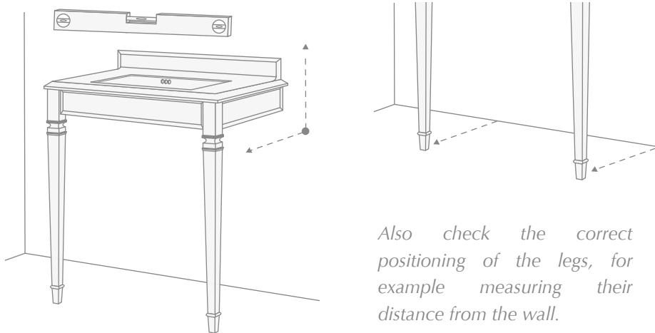
*Also check the correct positioning of the legs, for example measuring their distance from the wall.*
