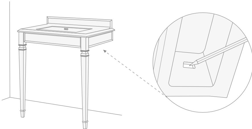
**10)** Remove the structure from the wall, drill the holes, place the rawlplugs and tighten the screws (G).
