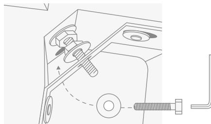
*Tighten the Allen screw using the Allen wrench without locking it definitively.*
