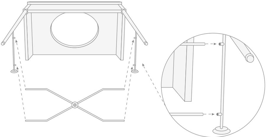
6) Temporarily fasten the cross to the legs with adhesive tape (if necessary protecting the part of the arms in contact with the tape).
