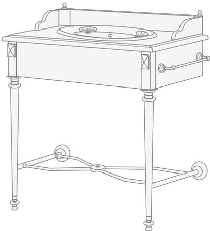
**17)** Slacken the screw fastening the shelf to the centre of the cross.
