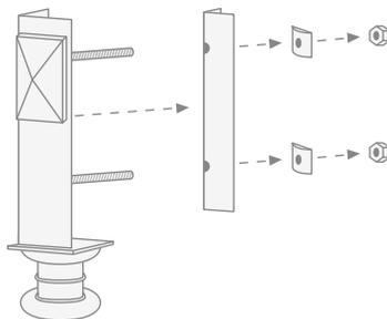
*Slacken the nuts and remove the spacers and internal plates inserted on the threaded bars in the top part of the leg.*
