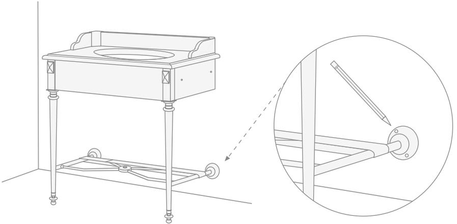
**9)** Mark the holes to fasten the wall support bracket (B). The bracket has an L-shaped section and must be positioned under the rear face of the top that is in contact with the wall.
