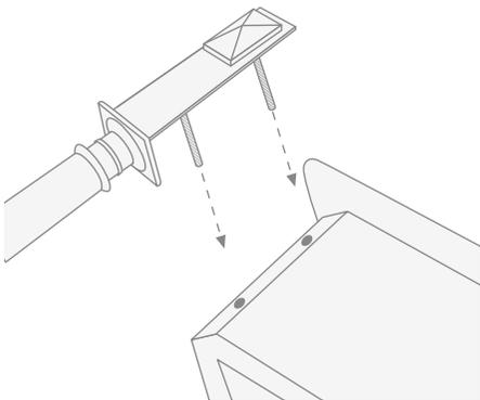
**3)** Move the leg into contact with the marble top, checking that both the threaded bars protrude from the inner part of the top.
