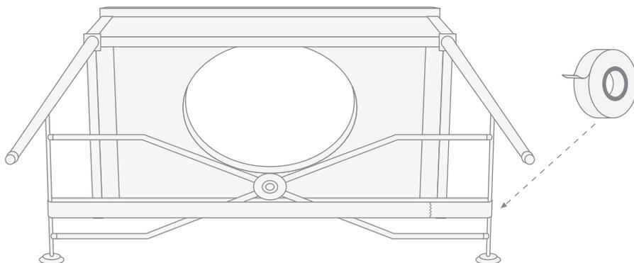
7) Lean the structure you have just assembled against the wall, making sure that it is positioned correctly by using a level in both a parallel and perpendicular position to the wall.
