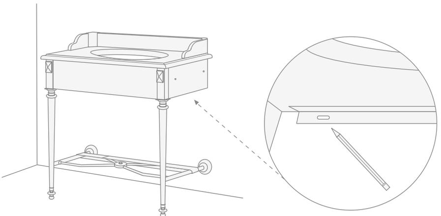
**10)** Remove the assembled structure from the wall and drill all the holes as marked.
