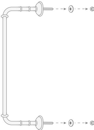
**12)** Insert the towel rail in its housing and fasten it tightening the bolts with their washers from the inner part of the marble top.
