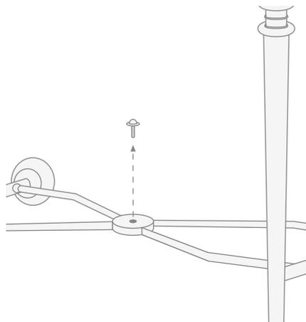
**18)** Position the glass shelf (C) and lock it with the centre screw.
