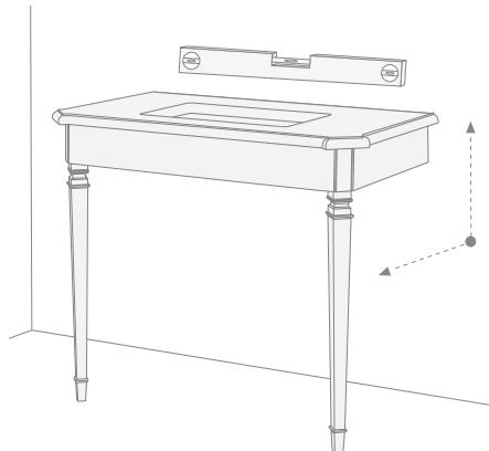
**11)** After finding the optimum position, mark the 2 points where holes need to be drilled to fix the console to the wall. Remove the console, drill the holes and insert the plugs (not supplied). Reposition the console against the wall and fix it into place with screws (not supplied).
