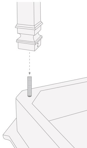
**5)** Fix the legs into position with the headless screws already inserted in the legs and with the Allen key (C).
