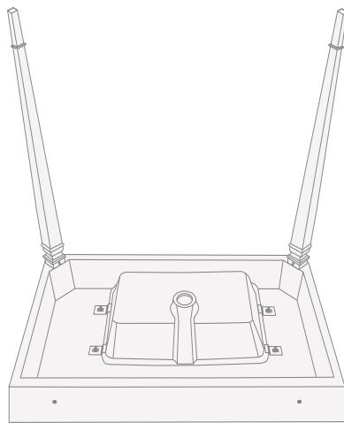
**10)** Turn the structure over and set it up against the wall, using a level to check the alignment parallel and perpendicular to the wall.
