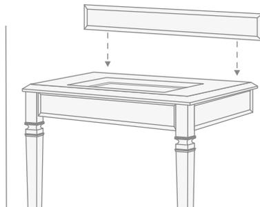
*Check precise positioning of the splashback before the silicone sets.*
