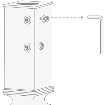
In the case of excess loosening of the one of the Allen screws and difficulty in retightening this, the cover on the top of the leg can be removed using a 17-mm pipe wrench. In this way, you can block the threaded metal plate inside the leg and retighten the Allen screw.
