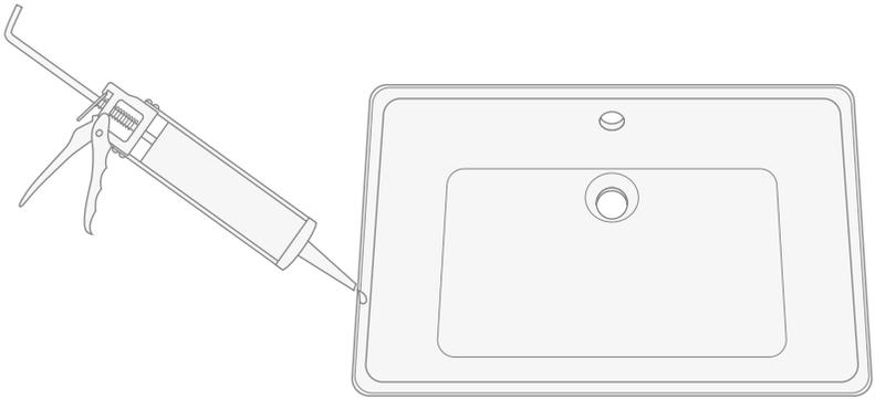
**14)** Position the basin on the unpolished surface of the marble counter and check correct positioning before the silicone sets.
