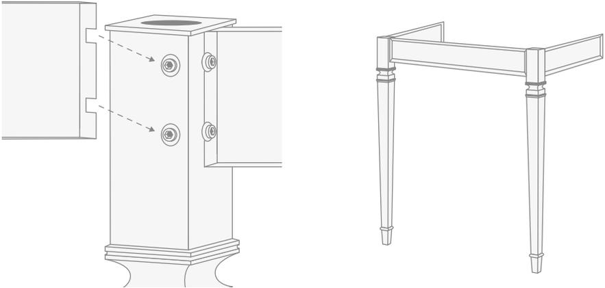
Lean the structure you have just assembled against the wall. Using a level, check that the structure is parallel and perpendicular to the wall.
