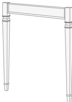
9) With the same procedure, fit the side panels. Note that only one end of the side panels has the U-shaped cuts. The other end has two holes for fastening to the wall.
