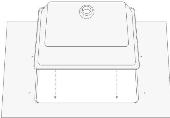
**15)** Fasten the basin to the top with the brackets (K), screws (L), bolts (M) and washers (N).
