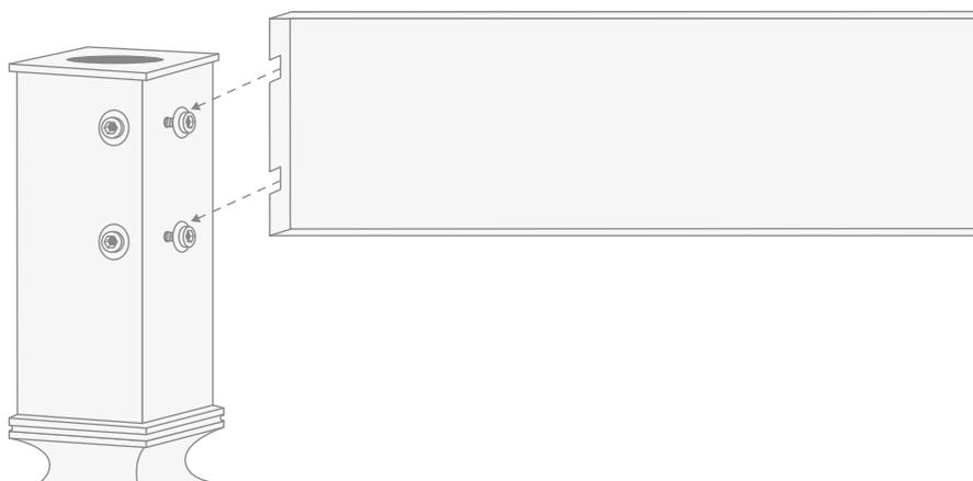
**7)** Tighten the Allen screws with the specific wrench.
