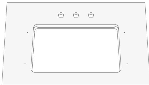
**13)** Apply a bead of silicon on the upper edge of the basin (J).
