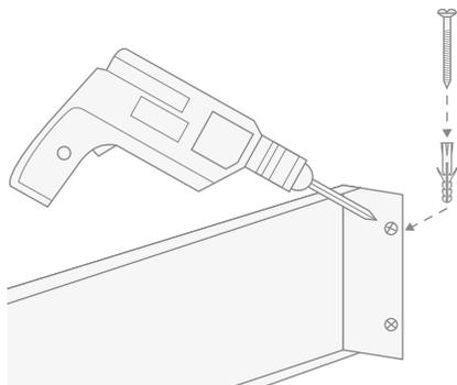
*Reposition the structure resting this on the wall and secure it with the screws provided.*
