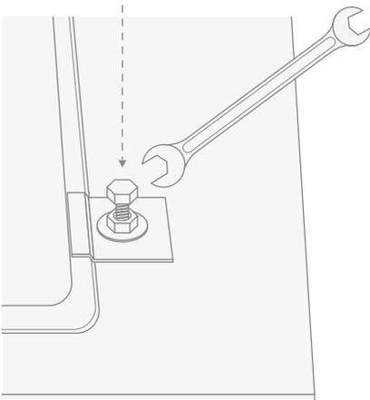
**17)** Position the top-basin structure above the structure fastened to the wall.
