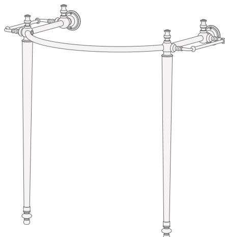
**8)** Set the structure in position against the wall and use a level to check its alignment parallel and perpendicular to the wall.
