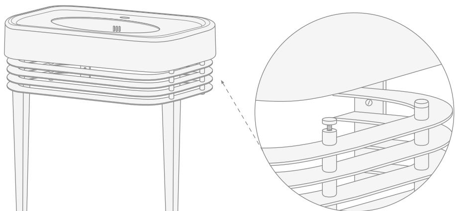
**10)** Check the final positioning of the washbasin using a level.
