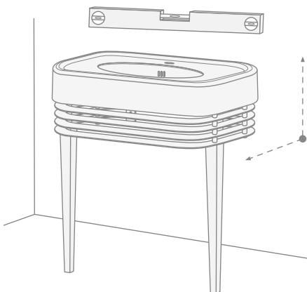
**11)** Mark out the 2 fixing holes on the wall for the washbasin. Remove the washbasin and create 2 holes using your pencil marks.
