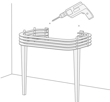
**12)** Insert the plugs provided into the holes. Put the washbasin in place again and fix it using the screws provided.
